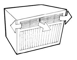
Air flow can also be directed up or down. Move the tab in the center louver in the desired air flow direction.
